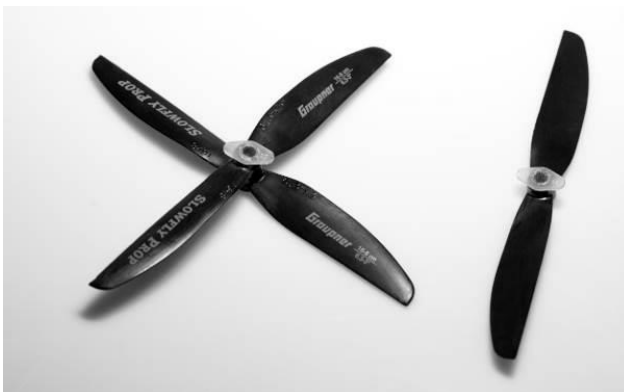
Fig. 1.5: Propellers 16 cm, 18 cm, 20 cm. (Inscription on the blade should be directed toward the generator)
