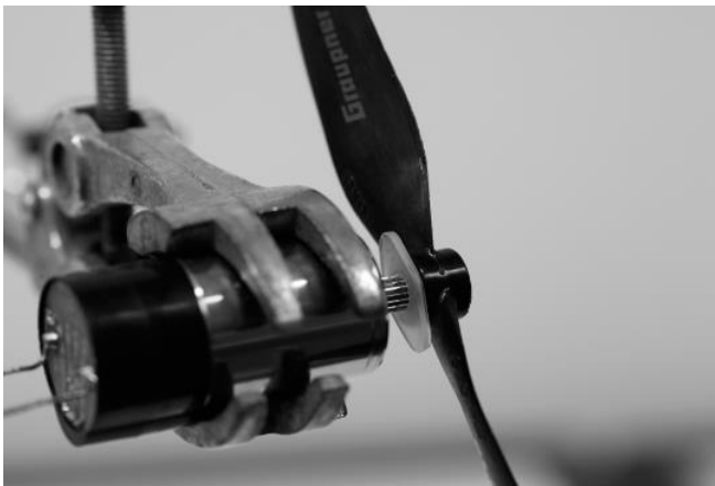
Fig. 1.8: Propeller mounted on the generator.
