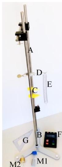
Figure 2 – 2 – Equipment used in 2 - 1.1: standing structure (A) mounted on a standing base (B), pointer pair (D), clamp with hook (C), spring (E), plastic tube with a suspending thread containing a pair of bar magnets (M1), brass mass (M2), stop watch (F) and square ruler (G).
